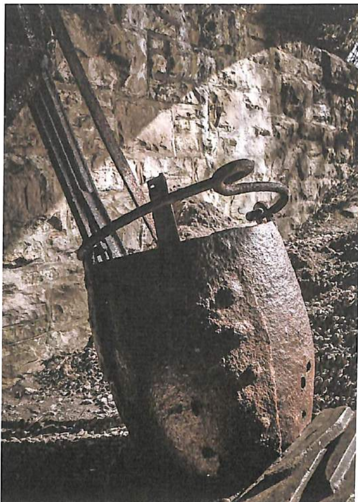
Lead Miner's Kibble used to lift material out of the mine, see article on Earby Mine Collection and Dales Countryside Museum's plans for this collection page 18.
