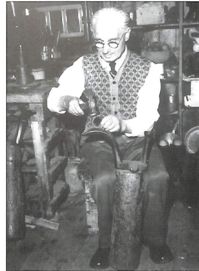
Photo: J V Brown, clogger at Airton, Malhamdale, using a clogger's stiddy – from the book "Making Boots, Shoes and Clogs" by Marie Hartley and Joan Ingilby.
